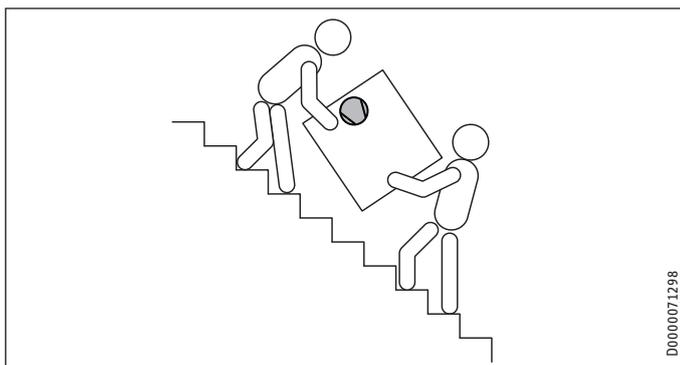
If the appliance needs to be tilted during transport, this must only be for a short time and it must only be tilted on one of its longitudinal sides. The longer the appliance is tilted, the greater the distribution of refrigerant oil inside the system.
